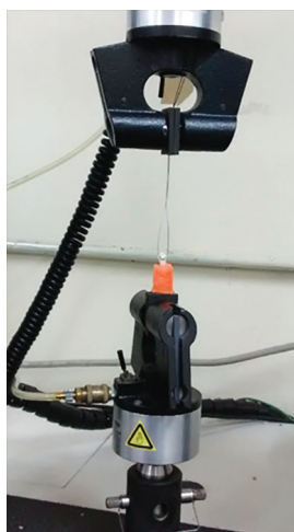
Fig. 4: Shear bond strength tested using universal testing machine
