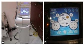
**Figs 1A and B:** (A) Er,Cr:YSGG laser (Biolase<sup>™</sup> Waterlase MD), (B) panel setting [1.25 W average power and 20 Hz (62.5 mJ/pulse)]
