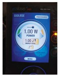
Fig. 6: Laser settings (Diode 940 mm, Ezlase, Biolase, USA)
