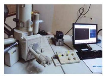
**Fig. 4:** Scanning electron microscope (JEOL. JSM-5600LV)
